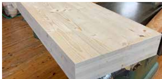
Prototype of 5-ply CLT with 100% re-used wood produced at NTI
